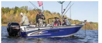
The 2000 Pro is designed for hardcore anglers with its full-vinyl bow and casting platforms, 24-volt prep for a trolling motor and 30-gallon aerated bow livewell to store the day's catch.
